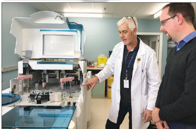
Medlab Central principal scientist Darrell Monk and DHB's Steve Carey with an analyser which can do approximately 50 different tests on one sample.
